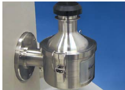
Cryo-Can connected to SEM chamber port
