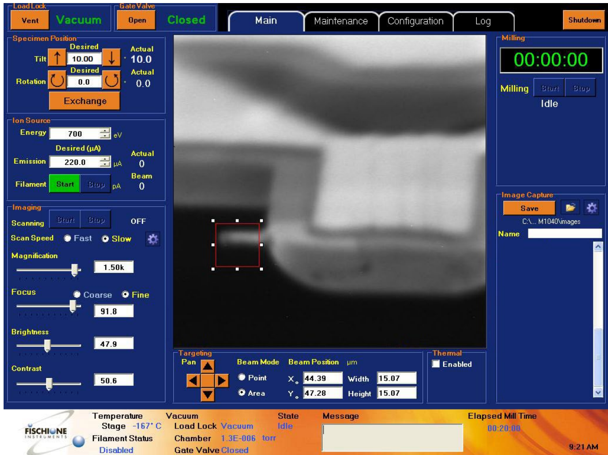
Figure 3. The secondary electron image shows the support grid and the lamella.
